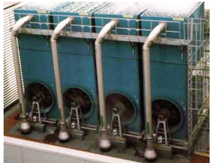
Marley CTF Series Cooling Tower —Forced draft, counterflow design. Fiberglass factory assembled modular structure. Film-fill or splash-fill option. Available in Europe only.
